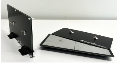
Fig. 2. The physical CPT system built from two identical PCBs.
