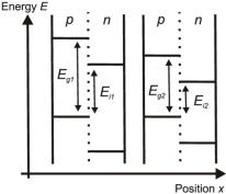
**Figure 2:** The schematic energy band diagram of a stacked organic tandem solar cell. The mutual position of the single cells does not matter, because the cells are only optically and not electrically in series. The absorber bandgap  $E_g$  and the interface bandgap  $E_i$  of each subcell are indicated.
