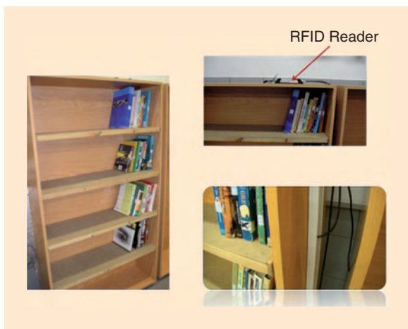
Figure 45. The prototype library cabinet with four shelves. The shelf antennas are fed on the side with coaxial cables running from the reader's ports or the multiplexer. Books (equipped with RFID tags) reside on top of the shelf antennas.
