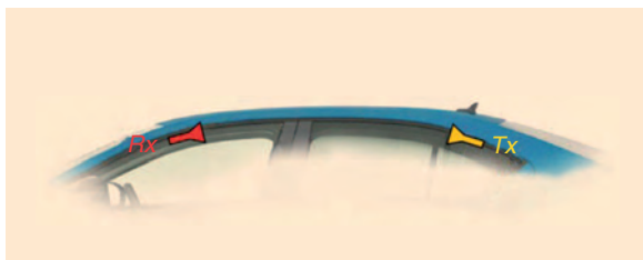
Figure 35. An experimental radio link that runs along the roof of a vehicle using a 3-D textile upholstery. Rx: receive; Tx: transmit.
